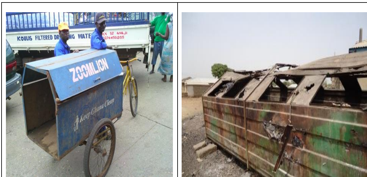
Figure 21: Spoilt lid Tricycle and a Burnt Refuse Container
