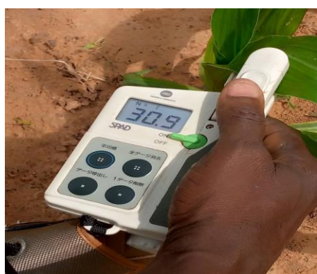
Figure 6. 5: Measuring chlorophyll content using a SPAD meter.
