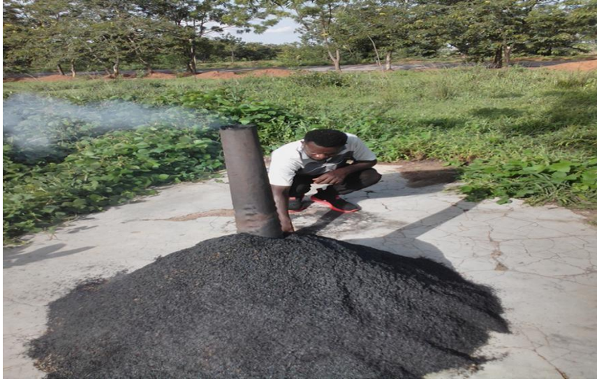
Figure 3.6. Production of rice husk Biochar using the pyrolysis method.
