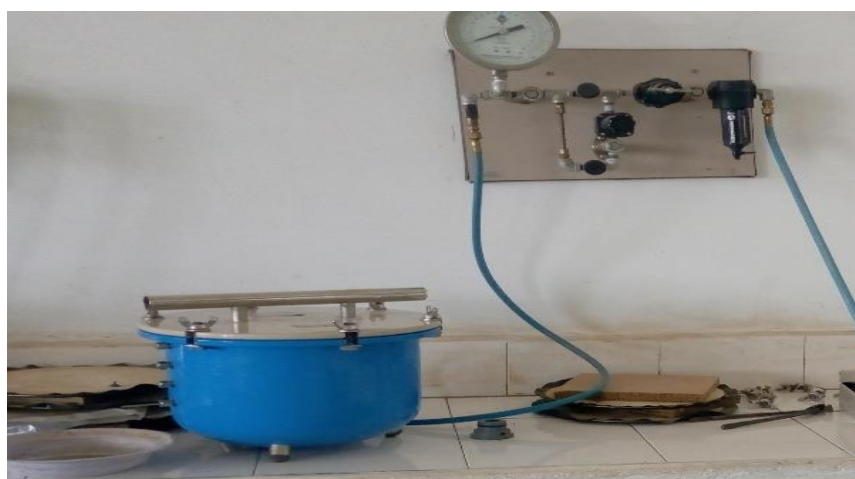
Plate 3.1: Laboratory Measurement of Field Capacity
