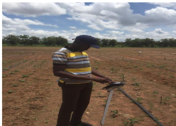
Appendix 29. Left: Data Collection on Okro, Right: Taking Data on Soil Moisture using Hydrosense II Soil Moisture Meter
