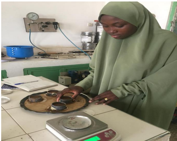
Appendix 32: Left: PWP and FC test in the laboratory; Right: Sample weighing for EC and P H tests
