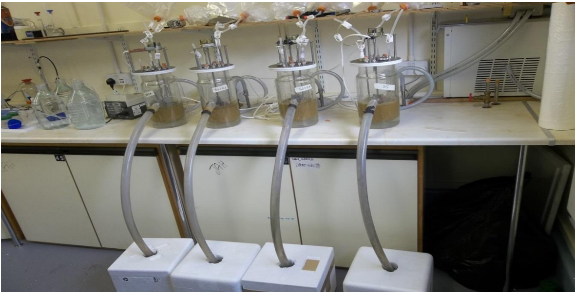
AP. 10 Vessels containing samples, gas collection bags, and other apparatus for the continuous culture experiment
