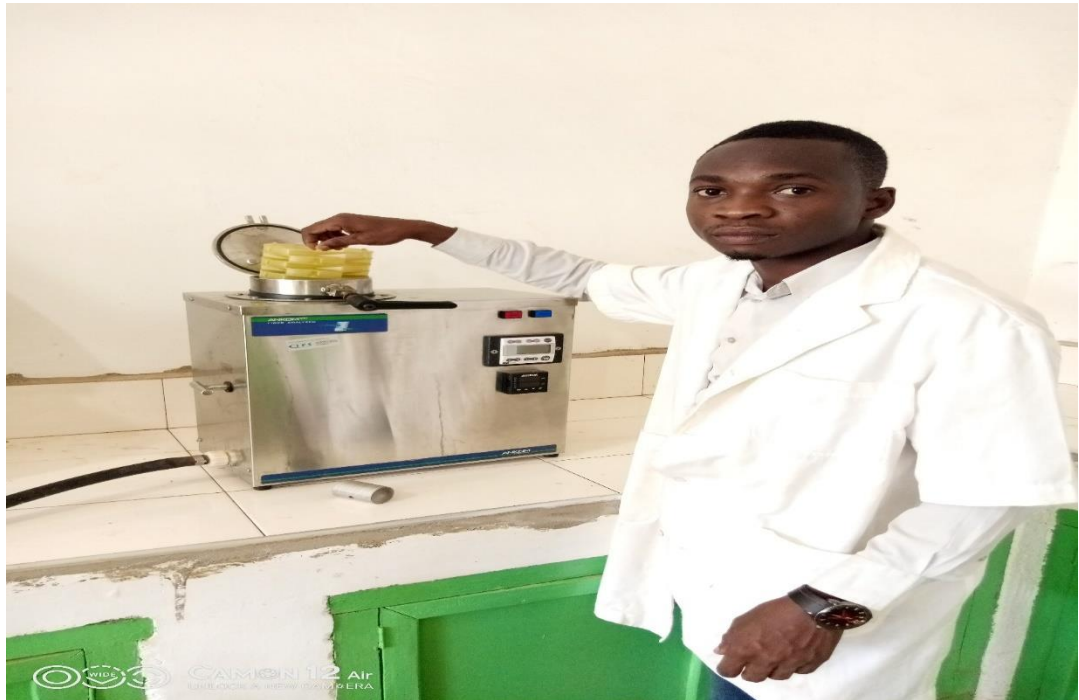
Plate 2. Determination of NDF and ADF with Ankom200 fibre analyser
