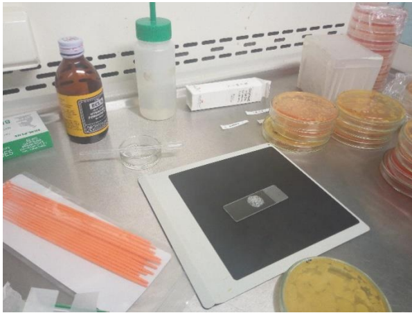
Plate 9: Set up for catalase test
