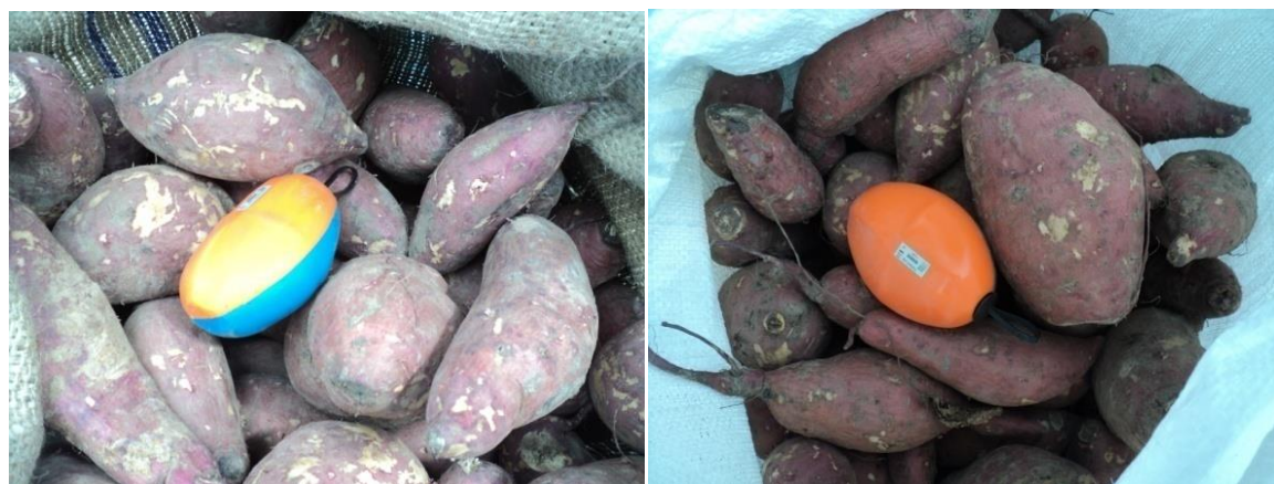
Plate 5: Impact data loggers inserted in sweetpotato storage root packages for transport to urban market.
