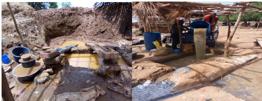
Plates 4.2 c and d: Washing of powdered ore to remove gold
