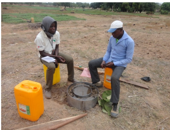
Plate 1: Infiltration test -upstream (Source: field studies, 2016)
