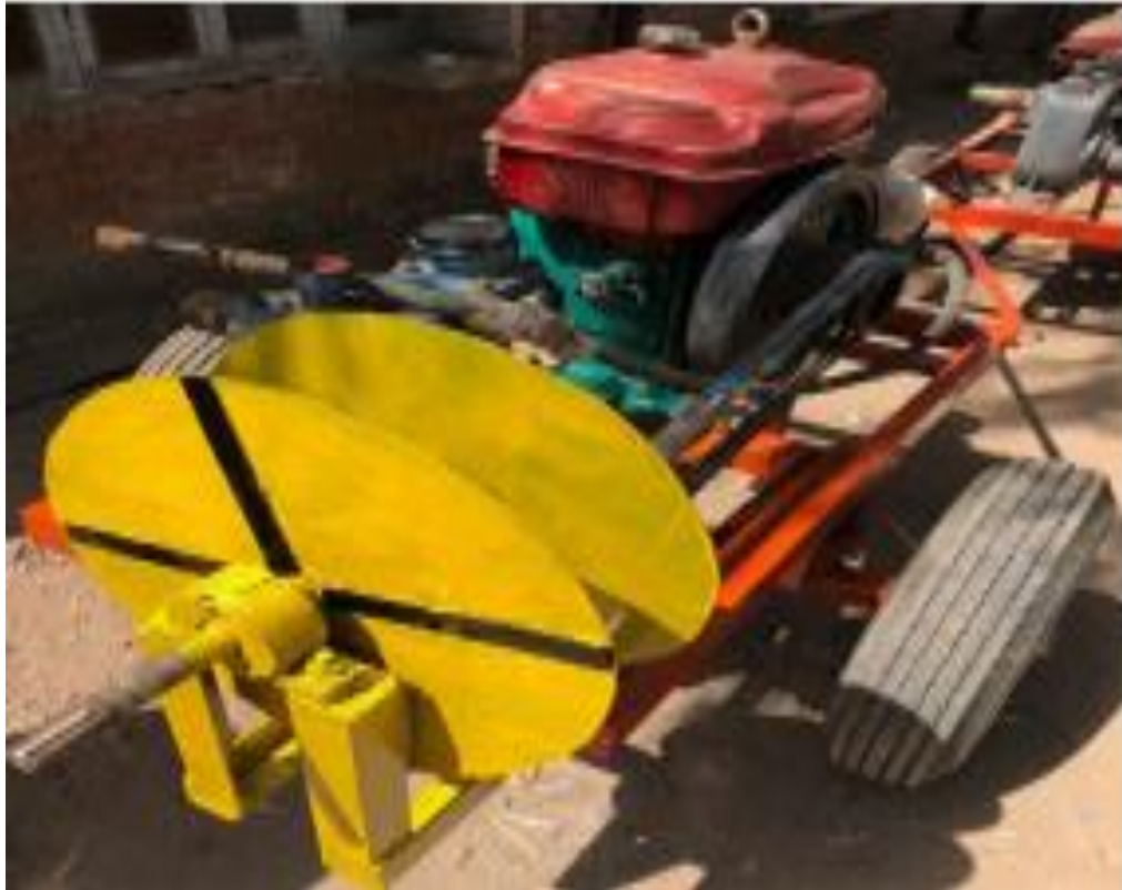
Figure 2. 7: Canvas pipe Hose reel Equipped with Mobile Sprinkler Rain Gun
