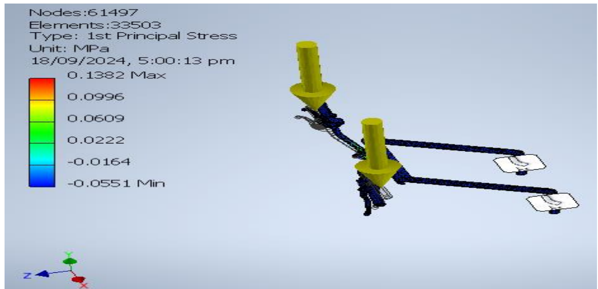
Figure 5.24: 1 st Principal Stress of the Control Bars
