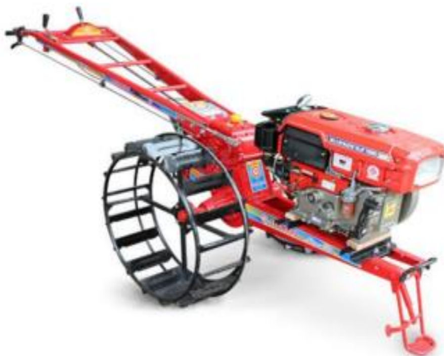
Figure 2. 5: Steel cage wheel Single Tool Tiller (Source: Rasool & Raheman, 2016)
