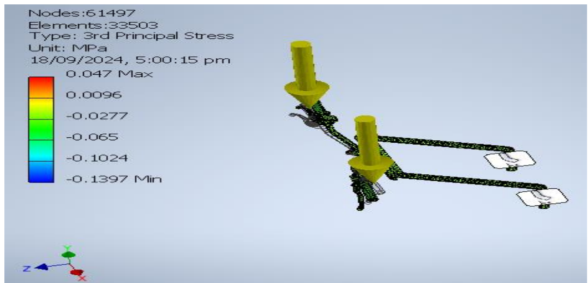
Figure 5.25: 3 rd Principal Stress of the Control Bars
