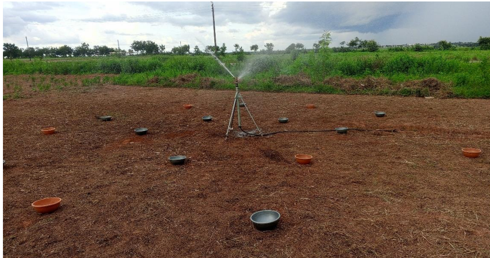
Figure 5.37: Collection of Water to Measure the Coefficient of Uniformity
