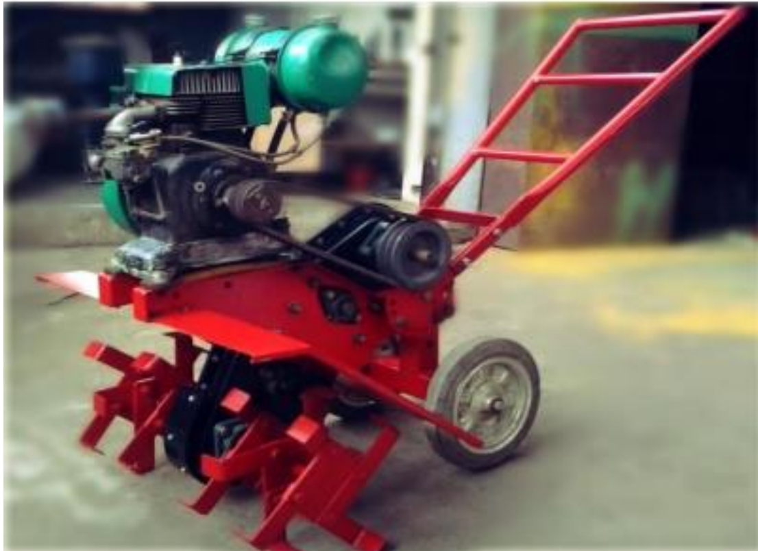
Figure 2. 6: Multi-Purpose Tiller (Source: Swapnil et al. , 2015)
