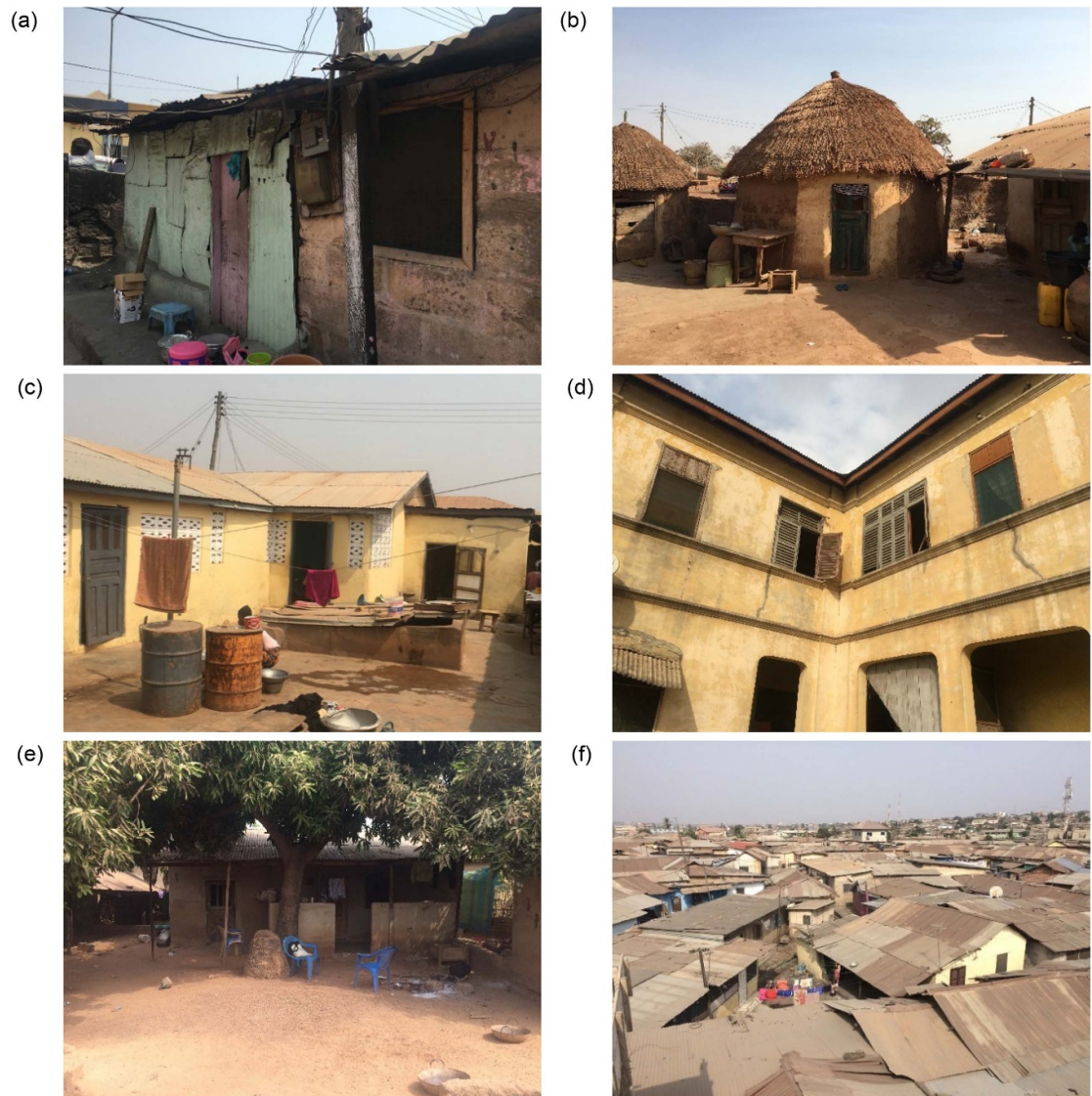
Figure 1. Example dwellings with: (a) wood walls and sheet metal-roof (Accra); (b) traditional mud walls and thatch roof (Tamale); (c) single-storey concrete block walls and sheet metal roof (Tamale); (d) two-storey/large concrete block walls (Accra); (e) some shade (Tamale); and (f) no shade (Accra).
