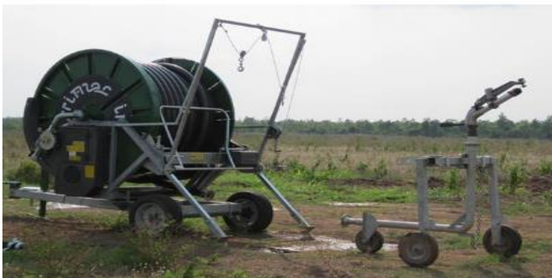
Plate2. 8: Hose-fed Traveling-Gun Sprinkler in Operation
