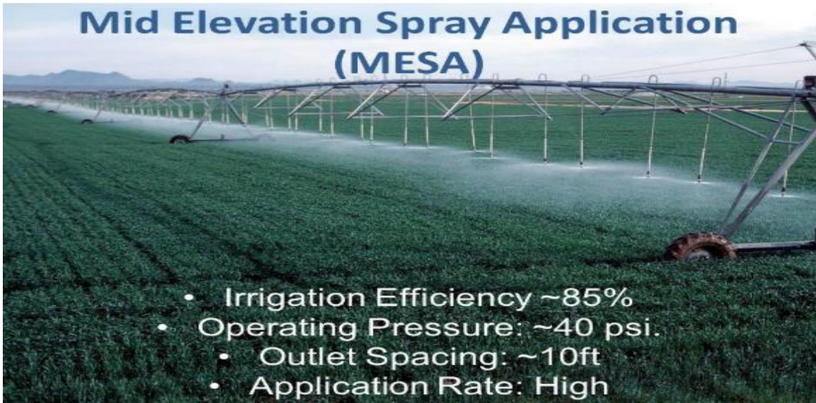
Plate2. 13: Mid Elevation Spray Application (MESA)
