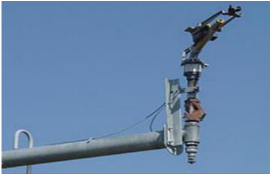
Plate2. 5: Part-circle Gun Sprinkler with Rocker Arm Drive.
