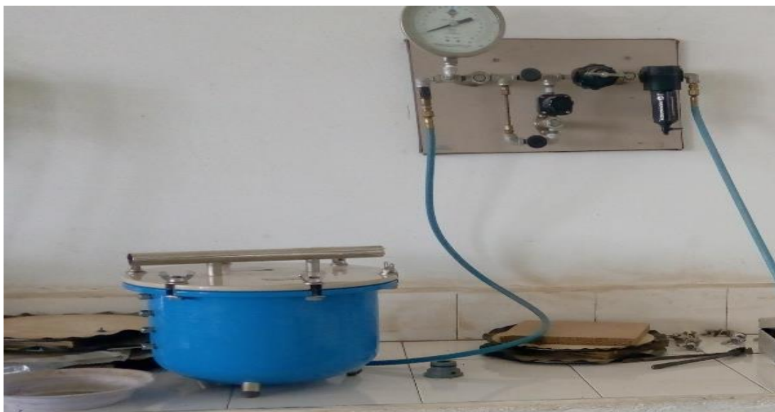
Plate3. 16: Determination of Field Capacity Using Pressure Plates
