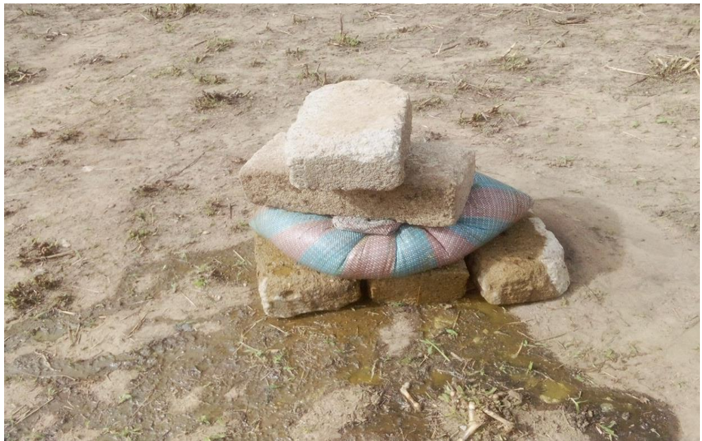
Plate 10: Expelling water to reduce the moisture content
