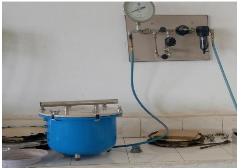
Plate 3.3: Determination of Field Capacity using Pressure Plates
