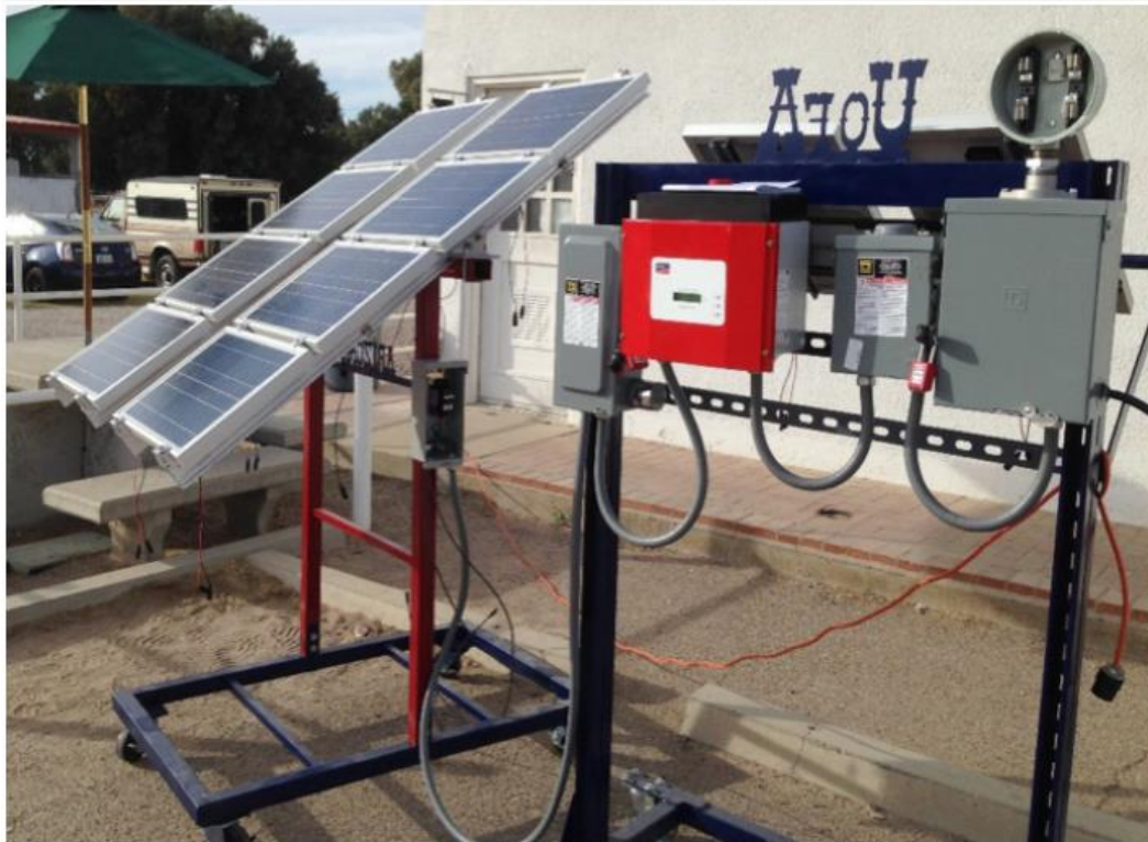
Figure 2.2: Grid Tied Solar System (Hybrid)
