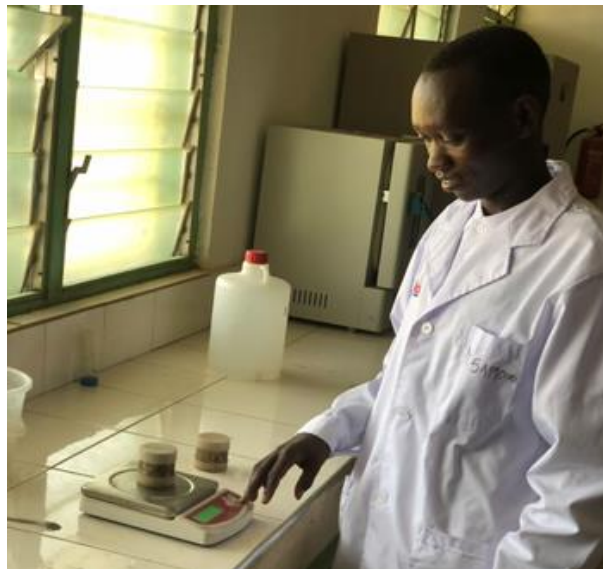
Plate 3.2: Measuring Soil Bulk Density at Laboratory
