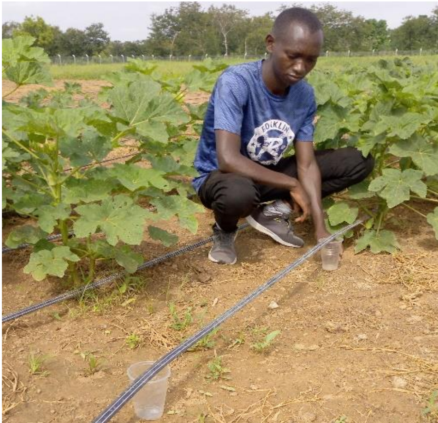
Plate 3.4: Catch Can Test for Drip Irrigation System at the WACWISA SPIS Site
