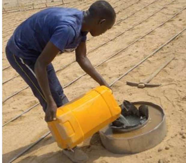
Plate 3.1: Measuring Infiltration Rate Using Double Ring Infiltrometer at the WACWISA SPIS Field
