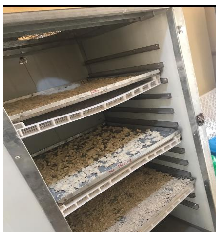
Plate 3.4: Electric drying of samples
