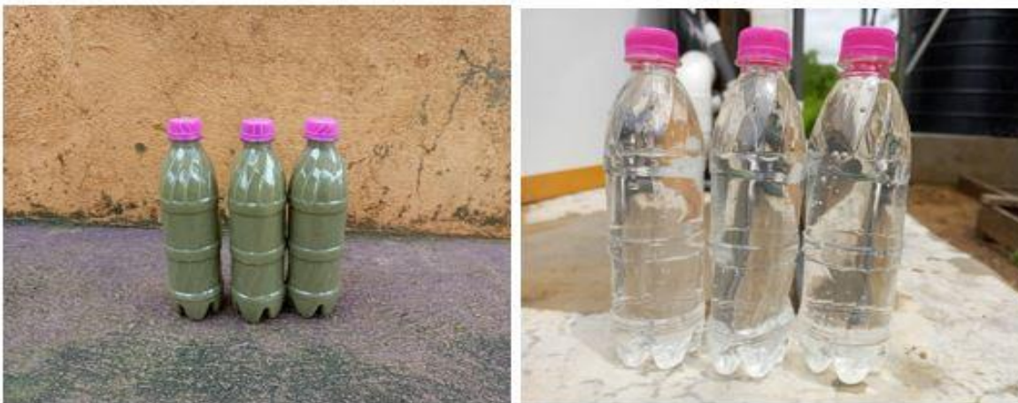
Figure 4: Visual Observation of Turbidity of Wastewater Sludge Before (left) and After (right) Filtration
