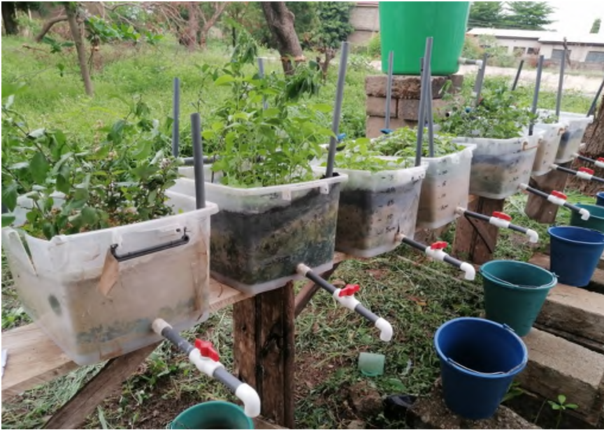
Figure 5: Experimental set up of the vertical flow CW with planted macrophytes
