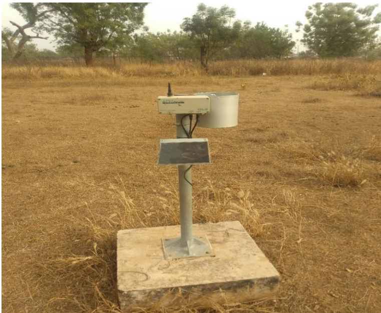
Figure 1: A community rain gauge at Kasuliyili.
