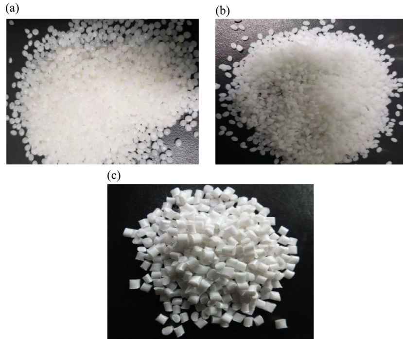
Figure 1 Examples of biodegradable polymers (BDPs) used as carbon sources in biofloc technology aquaculture systems: (a) Granules of polycaprolactone (PCL); (b) polybutylene succinate (PBS); (c) poly- \beta -hydroxybutyrate (PHB).
