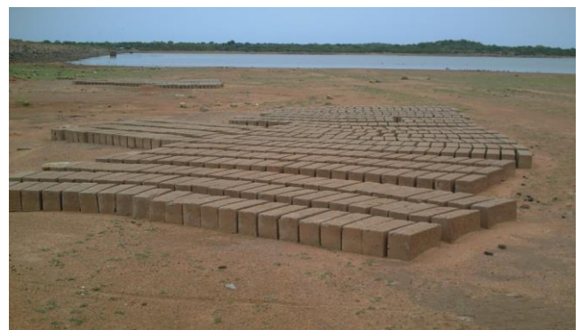
Plate 3: Building blocks made from the sand deposited in the Vea reservoir. The blocks are later carried to construction sites where they are used in the construction of buildings
