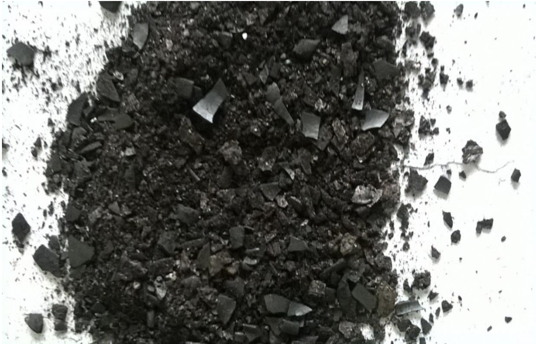
Plate 4: Shea nut shell biochar crushed for sieving through 2 mm standard sieve
