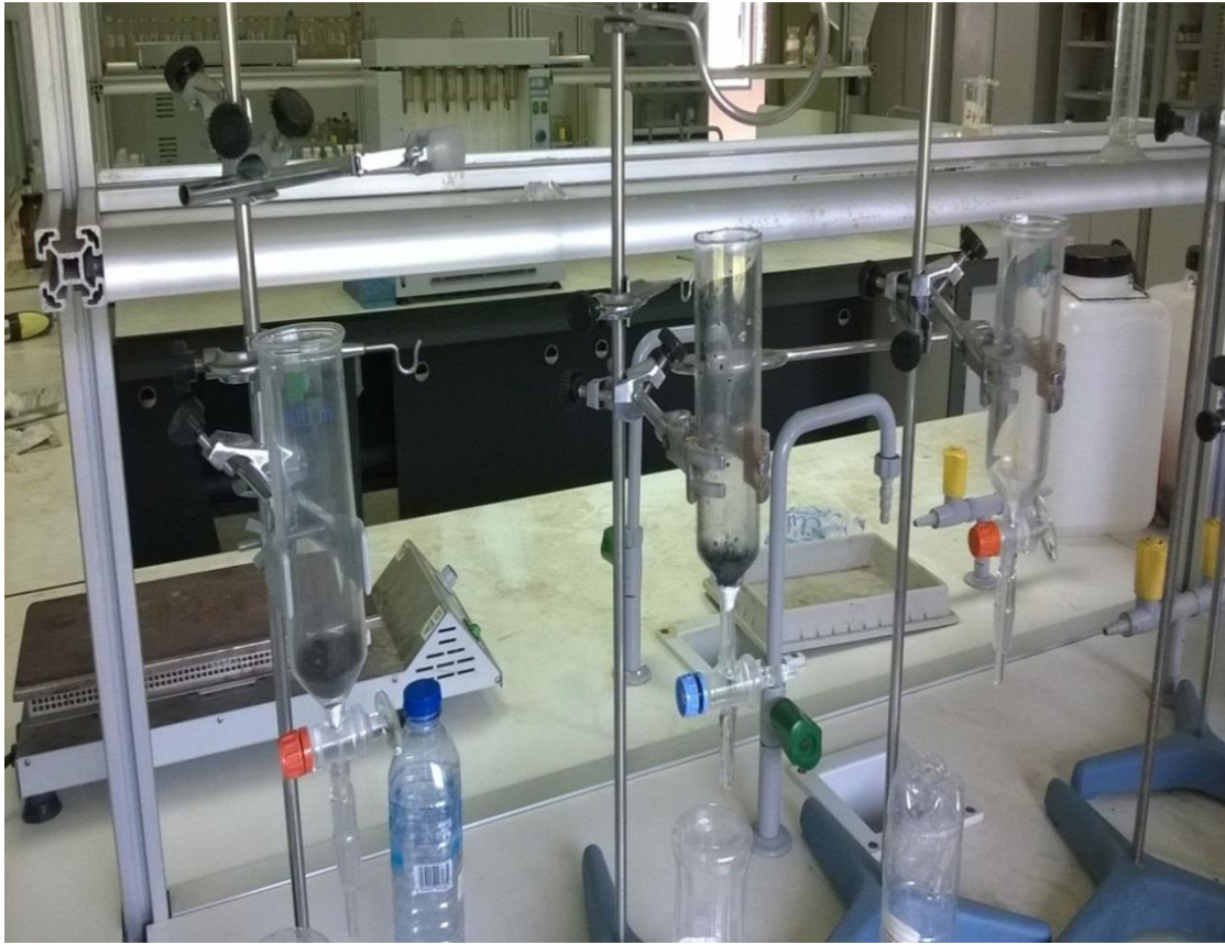
Plate 3: Separatory funnels with cotton wool and biochar
